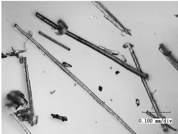
Figure 8 : sBF including fine particles obtained by grinding from SHS treated bamboo.
