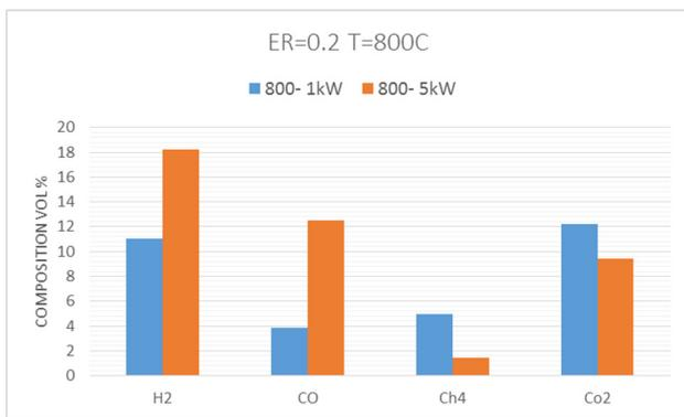
**Figure 8 :** Comparison of Syngas composition at 800°C for both reactors at equivalent ratio of 0.2
