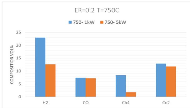
**Figure 7 :** Comparison of Syngas composition at 750°C for both reactors at equivalent ratio of 0.2
