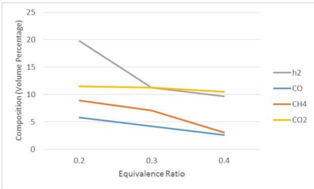
**Figure 3 :** The effect of Equivalence Ratio on gas compositions at 800°C in 1Kw gasifier
