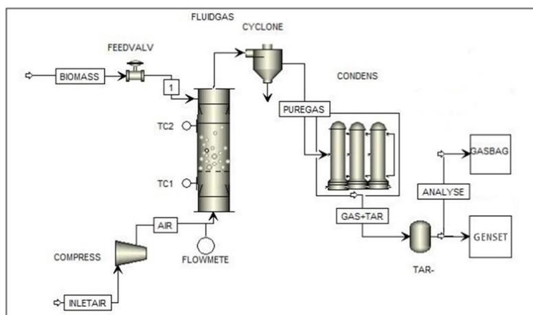
**Figure 2** : Schematic diagram of biomass air gasification in 5 kW fluidized bed reactor
