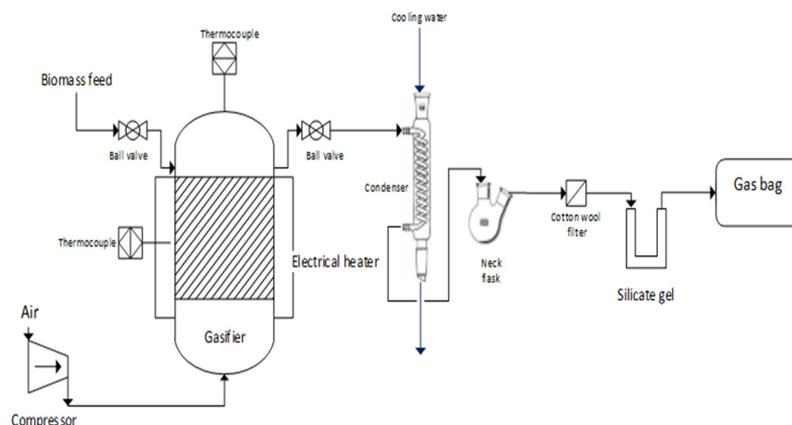
**Figure 1 :** Schematic diagram of biomass air gasification in 1 kW fluidized bed reactor
