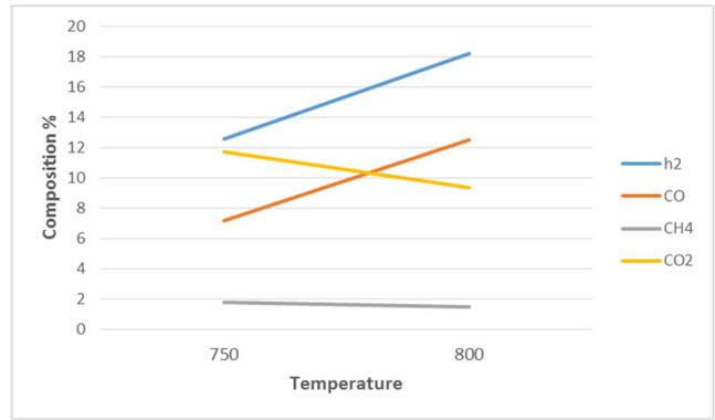
**Figure 5 :** The effect of temperature on Syngas composition in 5Kw gasifier
