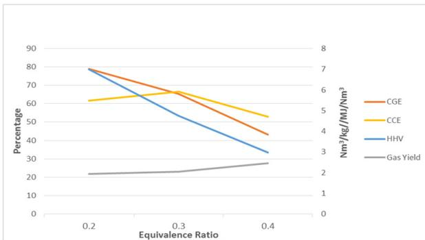
**Figure 4 :** The effect of Equivalence Ratio on carbon conversion efficiency, cold gas-efficiency, High heating value and gas yield in 1Kw gasifier
